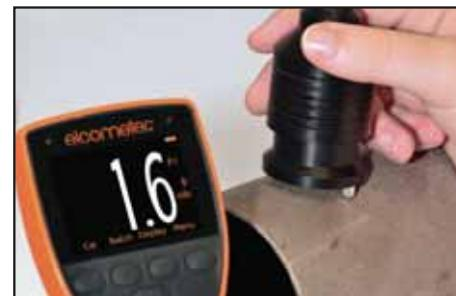
All Elcometer 224 Surface Profile Probes have an accuracy of  $\pm 5\%$  or  $\pm 5\mu\text{m}$  ( $\pm 0.2\text{mil}$ ) and are supplied with a glass zero plate, calibration test foils; nominal values 125 $\mu\text{m}$  (5.0mils) & 508 $\mu\text{m}$  (20mils) and an Elcometer test certificate.
